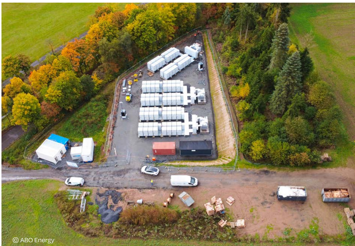
Waldkappel Battery Park, Waldkappel, Hesse, Germany — 16 MW / over 33 MWh stand-alone battery energy storage system
